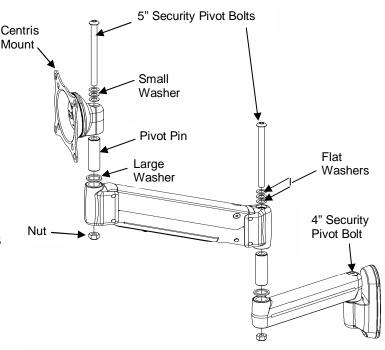
Figure 5. Install 5-inch Security Pivot Bolt (Lift Arm Example)
